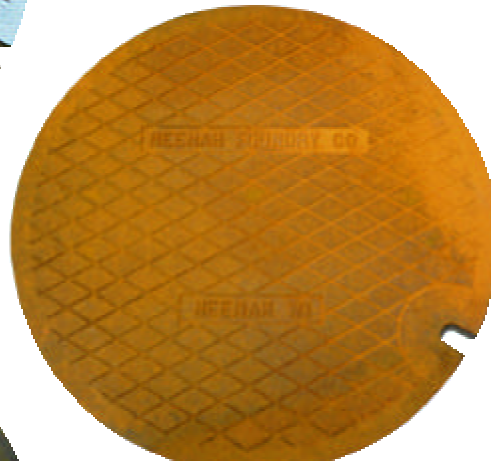
Figure 3 Full surface oxidation after complete wetting
